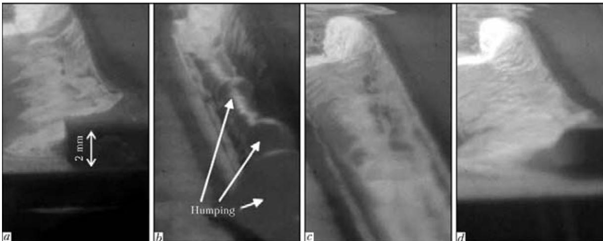
**Figure 9.** Influence of shielding gas on humps formation in overlap joint (steel S420MC 2 mm thick,  $v_w = 10$  m/min, shots behind the welding process):  $a, b$  – without shielding gas;  $c, d$  – with Ar + O<sub>2</sub> gas
