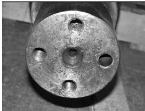
Figure 9. Repaired channel for thread cutting
