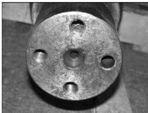
**Figure 9.** Repaired channel for thread cutting
