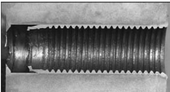
**Figure 5.** Macrosection of repaired threaded opening
