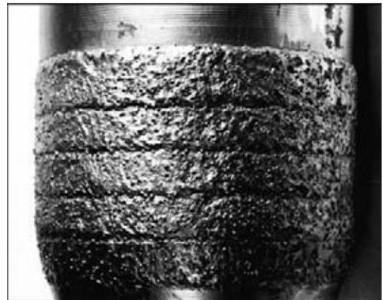
Drill pipe lock cladded by spherical tungsten carbide
