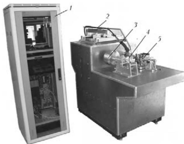
**Figure 2.** General view of machine MIS for HC testing on the RF standard: 1 – box for control of test parameters, their imaging and registration; 2 – manipulator of welding head for its movement along  $x$ ,  $y$  and  $xy$  axes; 3 – force measure device; 4 – machine for welding of samples and their bending or tensile tests; 5 – machine for simulation of welding cycle in the samples and HC tests at cooling stage
