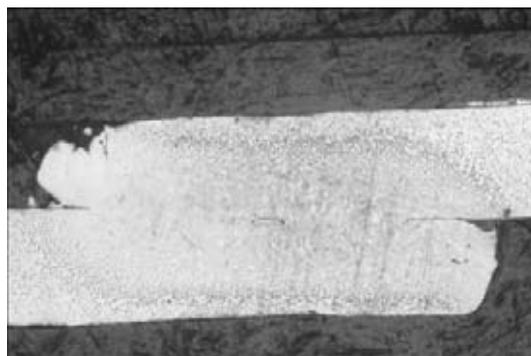
**Figure 6.** Macrosection ( $\times 50$ ) of braze-welded joint across the section near the joint center
