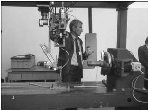
Demonstration of possibilities of 3D portal manipulator, equipped by the TRUMPF optical head with irradiation scanning system
