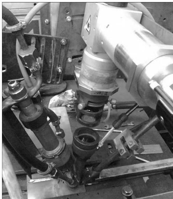
**Figure 2.** Appearance of the welding head for laser-arc welding of titanium alloys
