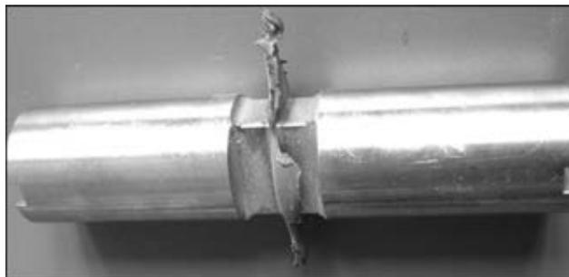
Figure 3. LF welded joint on titanium alloy (specimen is supplied by The Welding Institute, Great Britain)
