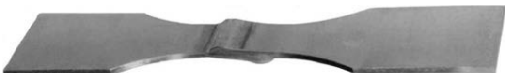
Figure 3. Sample of overlap joint for fatigue testing
