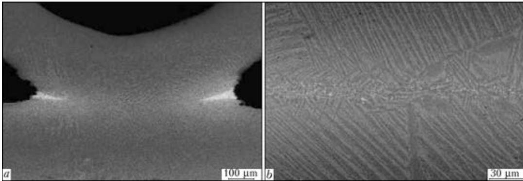
**Figure 8.** Microstructures of brazed fragment of the lamellar-ribbed titanium heat exchanger: *a* – general view of the joint with fillet regions; *b* – central zone of the seam
