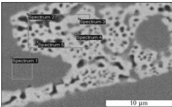
**Figure 5.** Microstructure of eutectic region of the brazed seam made by using filler alloy with the crystalline structure
