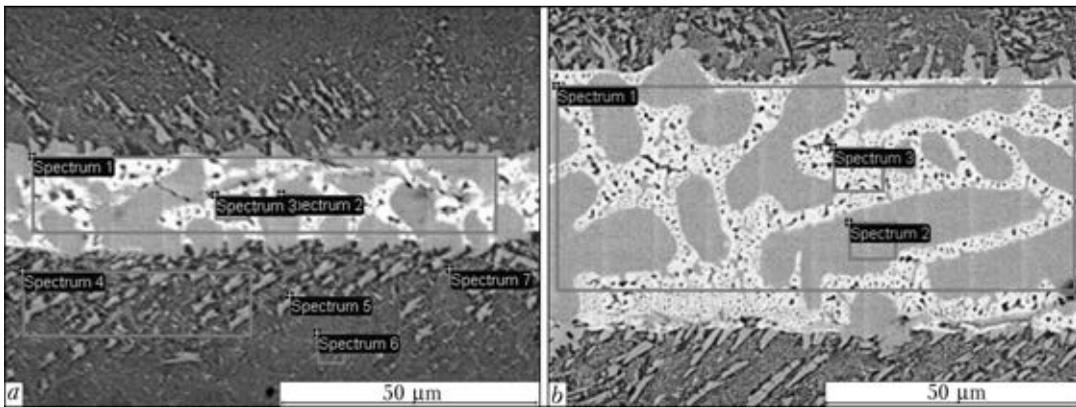
**Figure 4.** Microstructure of region of the brazed seam made by using filler alloy with the amorphous (*a*) and crystalline (*b*) structure
