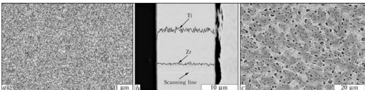
**Figure 2.** Microstructures of filler alloy in the amorphous (*a*) and crystalline (*c*) states, and character of distribution of alloying elements in the amorphous filler alloy (*b*)
