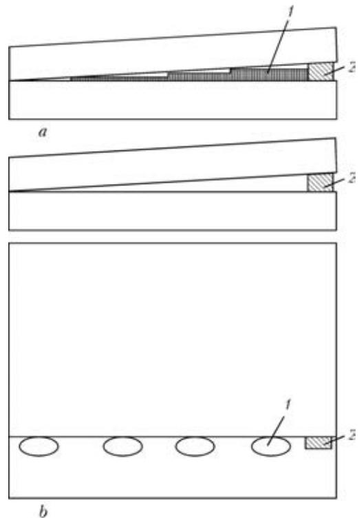
**Figure 1.** Schematics of samples for conducting metallographic examinations using filler alloy in the amorphous (*a*) and cast (*b*) states: 1 – filler alloy; 2 – inserted element for fixation of gap
