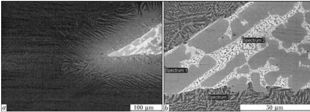
**Figure 3.** Microstructures of the reverse (*a*) and direct (*b*) fillets of the brazed joint made by using filler alloy with the crystalline structure
