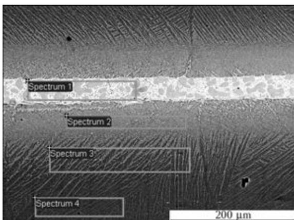
**Figure 7.** Microstructure of the joint brazed with the amorphous filler alloy
