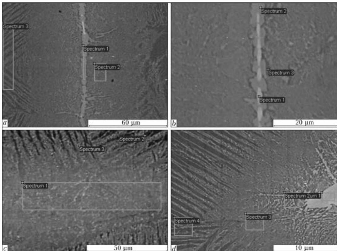
**Figure 6.** Microstructures of the seams made with decrease in the brazing gap by using filler alloy with the amorphous (a, c) and crystalline (b, d) structure
