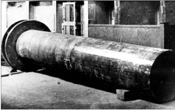
**Figure 5.** Mould for vacuum electric-arc melting titanium ingots of bronze BrKh08 40 mm thick
