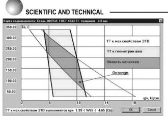
**Figure 8.** Plotting of the quality region in optimisation of thermal parameters of welding in software «System for Computer Analysis of Weldability of Steels»
