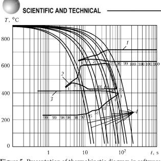
**Figure 5.** Presentation of thermokinetic diagram in software «Sysweld/Visual-Weld»: *1*–*4* – phases 1–4, respectively
