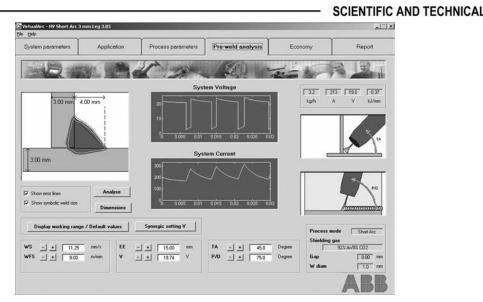
Figure 9. «Virtual ARC» software window
