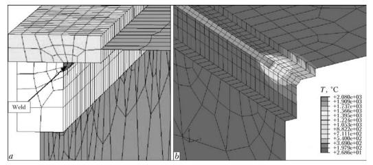
**Figure 6.** Software «Abaqus»: a - finite element model of weldment; <math>b - finite element fields
