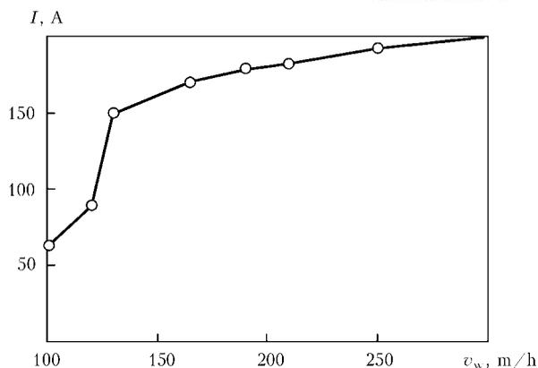
**Figure 2.** Dependence of speed of hybrid welding of alloy AMg6 2 mm thick on arc current at input of emission power of CO<sub>2</sub>-laser of 2.8 kW into metal [10]
