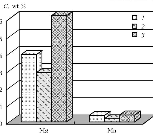
**Figure 4.** Effect of energy input  $E$  of laser welding of alloy AMg6 ( $\delta = 1.2$  mm) at density of emission power  $W = 2 \cdot 10^7$  W/cm<sup>2</sup> on content of alloying elements  $C$  in weld cast metal: 1 – laser welding,  $E = 50$ ; 2 – laser welding,  $E = 120$  J/mm; 3 – base metal
