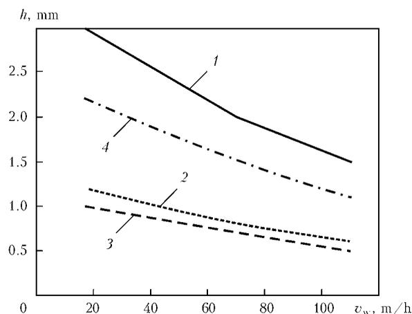
**Figure 3.** Dependence of penetration depth on speed of welding the aluminium alloy AMg6 ( $\delta = 1-3$  mm): 1 – hybrid laser-plasma welding; 2 – laser welding; 3 – plasma welding; 4 – sum of depths of penetrations obtained by laser and plasma welding ( $P_L = 1.2$  kW;  $I_{SP}/I_{RP} = 50/50$  A;  $U_a = 18$  V)
