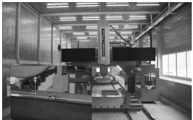
Figure 7. Weld monitoring at the gantry center HAGE-MATIC 305 FSW for processing using cutting and FSW
