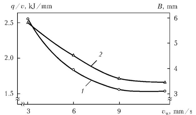
**Figure 3.** Dependence of energy input (1) and width of face weld bead (2) on speed of welding of steels 10Kh12M and 10Kh9MFBA of  $\delta = 30$  mm in flat position at  $U_{acc} = 60$  kV,  $-\Delta I_f = 15$  mA,  $d_{circ} = 1.5$  mm and  $l_{work} = 200$  mm
