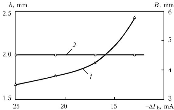
**Figure 6.** Dependence of width of face (1) and reverse (2) weld beads on deepening of electron beam focus in EBW of heat-resistant steels 10Kh12M and 10Kh9MFBA 30 mm thick using horizontal beam at  $U_{acc} = 60$  kV,  $I_b = 198$  mA,  $v_w = 6$  mm/s,  $d_{circ} = 1.5$  mm and  $l_{work} = 200$  mm
