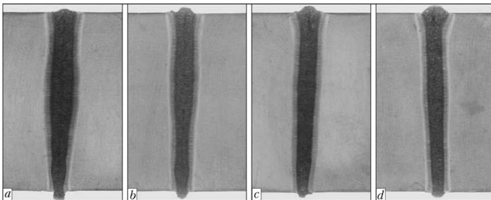
**Figure 4.** Macrostructure ( $\times 2$ ) of welded joints on 10Kh12M alloy of  $\delta = 30$  mm in welding using horizontal beam at  $U_{acc} = 60$  kV,  $I_b = 198$  mA,  $v_w = 6$  mm/s,  $d_{circ} = 1.5$  mm and  $l_{work} = 200$  mm:  $a\text{--}d$  – respectively,  $-\Delta I_f = 25, 21, 17$  and 13 mA
