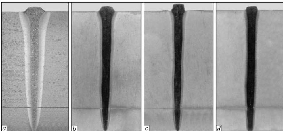
**Figure 2.** Macrostructure ( $\times 1.5$ ) of welded joints on 10Kh9MFBA alloy of  $\delta = 30$  mm in flat position at  $U_{acc} = 60$  kV,  $I_f = 630$  mA,  $-\Delta I_f = 15$  mA,  $d_{circ} = 1.5$  mm,  $l_{work} = 200$  mm (*a-d* –  $v_w$  and  $I_b$  are the same as in Figure 1)
