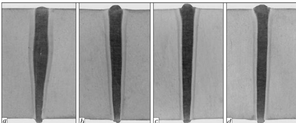
**Figure 5.** Macrostructure ( $\times 2$ ) of welded joints on 10Kh9MFBA alloy of  $\delta = 30$  mm in welding using horizontal beam ( $U_{acc}$ ,  $I_b$ ,  $v_w$ ,  $d_{circ}$ ,  $l_{work}$  and  $a\text{--}d$  are the same as in Figure 4)
