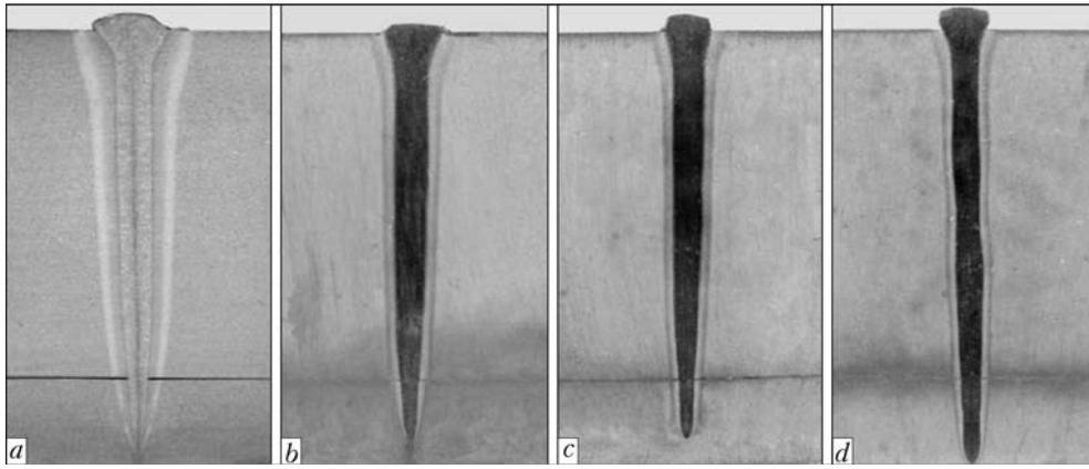
**Figure 1.** Macrostructure ( $\times 1.5$ ) of welded joints on 10Kh12M alloy of  $\delta = 30$  mm in flat position at  $U_{acc} = 60$  kV,  $I_f = 630$  mA,  $-\Delta I_f = 15$  mA,  $d_{circ} = 1.5$  mm,  $l_{work} = 200$  mm: *a* –  $v_w = 3$  mm/s,  $I_b = 128$  mA; *b* –  $v_w = 6$  mm/s,  $I_b = 184$  mA; *c* –  $v_w = 9$  mm/s,  $I_b = 236$  mA; *d* –  $v_w = 12$  mm/s,  $I_b = 310$  mA
