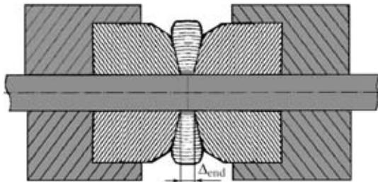
**Figure 4.** Scheme of formation of welded joint with end gap  $\Delta_{end}$
