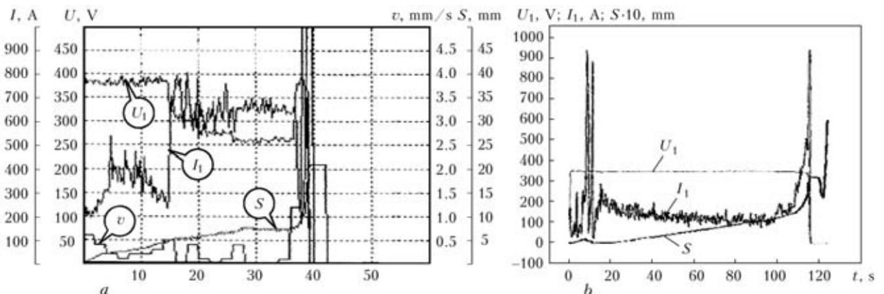
Figure 3. Program of change of main parameters of process in welding of aluminium alloy parts of cross section area 30 × 140 mm by pulsating (a) and continuous (b) flashing
