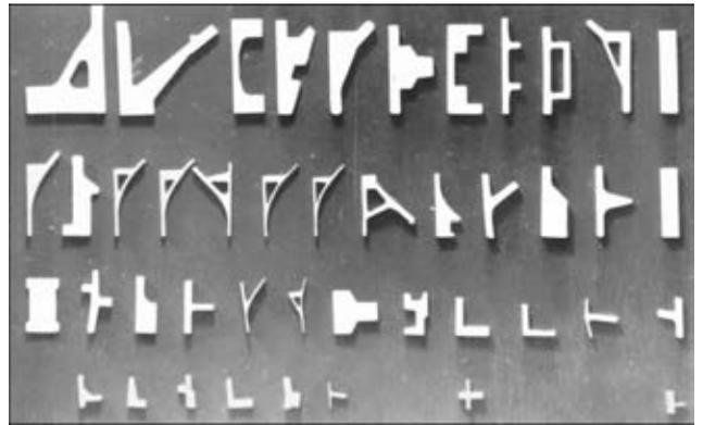
Figure 1. Examples of aluminium alloy profiles welded by FBW
