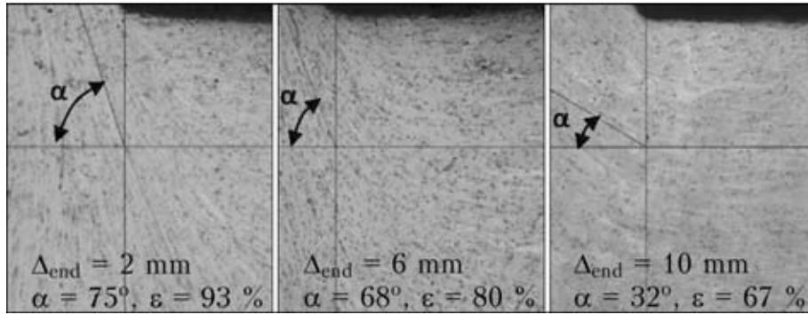
**Figure 6.** Macrostructures of zone of welded joint (a-c) in welding alloy 1201 of 30 mm thickness at different final degree of deformation
