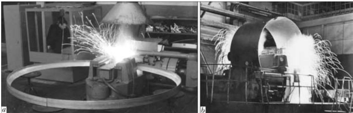
Figure 2. FBW of frame rings in machine K393 (a) and shells in machine K767 (b)
