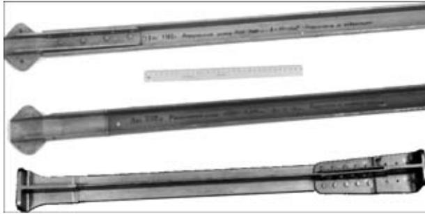
**Figure 9.** Riveted and welded joint of dissimilar alloys on aluminium base of fitting–stringer elements used in aerospace industry
