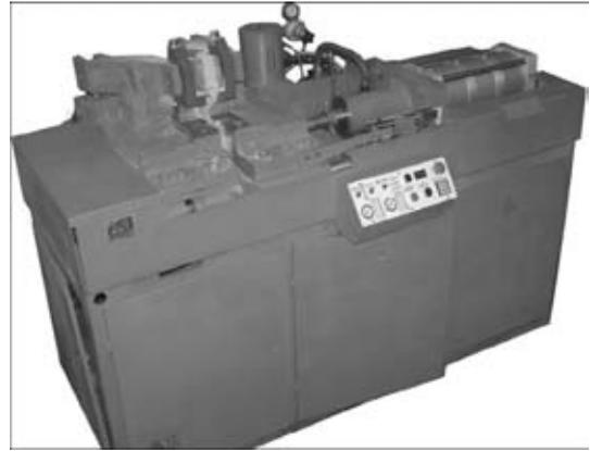
**Figure 10.** Machine for FBW of thin-wall profiles of high-strength aluminium alloys
