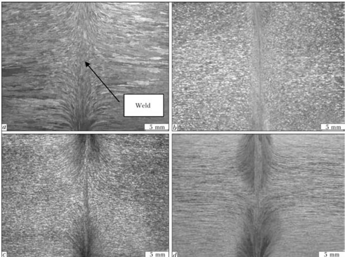
**Figure 8.** Macrostructures of welded joints of alloys 1201 (a), AD33 (b), 1570 (c) and V95 (d) made by FBW
