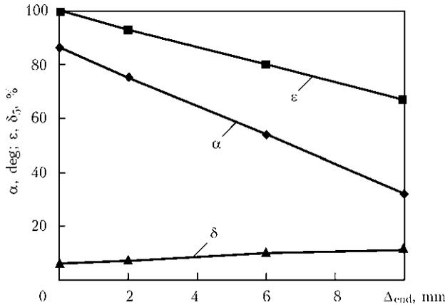
**Figure 5.** Dependence of deformation degree, bending angle of fiber and elongation on end gap
