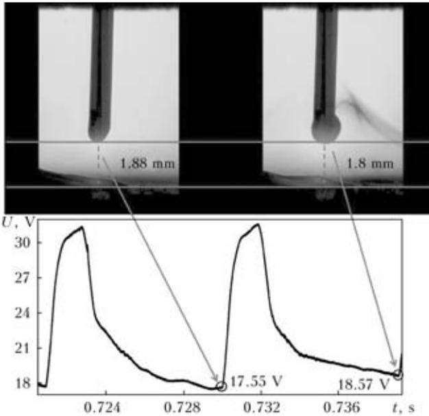
**Figure 1.** Non-proportionality of geometrical arc length and welding voltage
