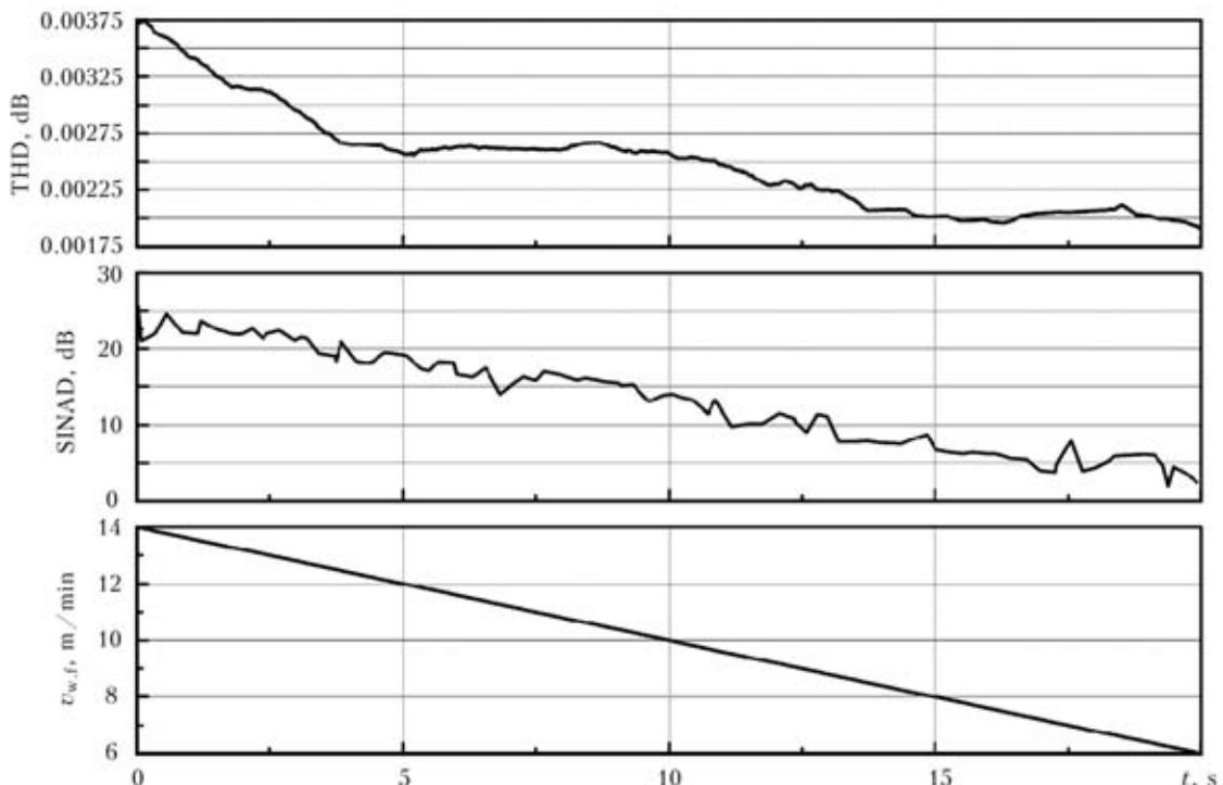
**Figure 7.** THD and SINAD versus wire feed rate
