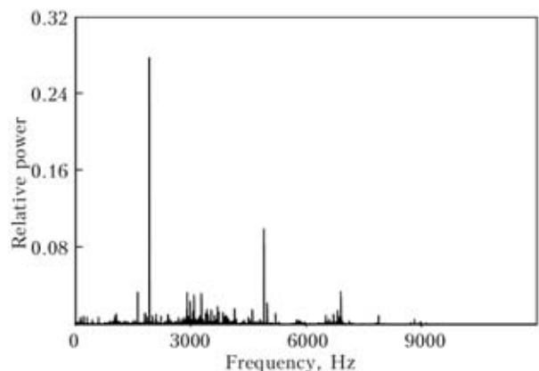
**Figure 3.** Spectrum of triad coupled into inverter power source
