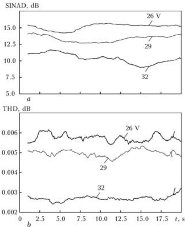
**Figure 5.** Chronological sequence of SINAD (a) and THD at welding voltage of 26, 29 and 32 V
