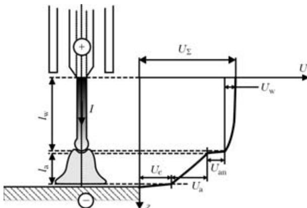
**Figure 2.** Operative path of arc welding process with idealised potential curves
