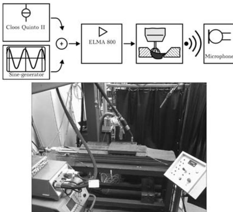
Figure 4. Test set-up of welding equipment
