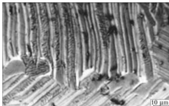
**Figure 8.** Microstructure of brazed joint of titanium aluminide obtained using BFM of Ti–Zr–Fe system with cast structure
