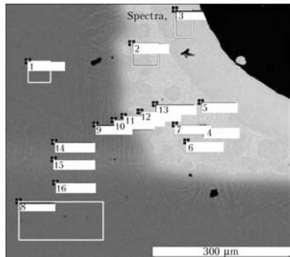
**Figure 4.** Microstructure and areas of X-ray microspectrum analysis of brazed joint (OT4 base metal, Ti-Zr-Co BFM)
