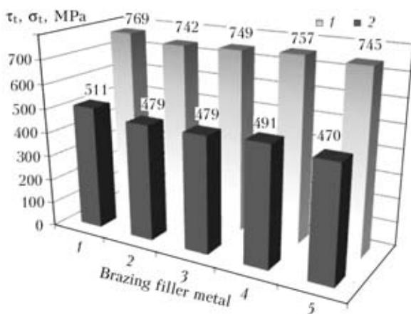
**Figure 7.** Tensile strength of brazed butt  $\sigma_t$  (1) and lap  $\tau_t$  (2) specimens (base metal VT6) obtained using BFMs on the basis of systems: 1 – Ti–Zr–Co; 2 – Ti–Zr–Cu–Ni; 3 – Ti–Zr–Cu–Ni; 4 – Ti–Zr–Fe; 5 – Ti–Zr–Fe
