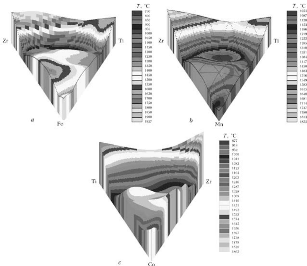
**Figure 1.** Liquidus surface of alloys of Ti-Zr-Fe (a), Ti-Zr-Mn (b) and Ti-Zr-Co (c) systems
