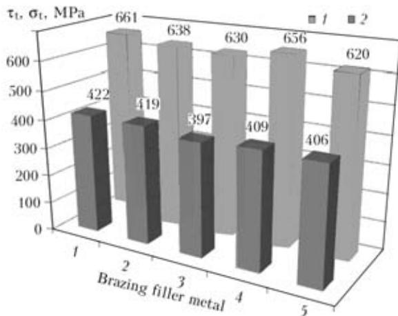
**Figure 6.** Tensile strength of brazed butt  $\sigma_t$  (1) and lap  $\tau_t$  (2) specimens (base metal OT4) obtained using BFMs on the basis of systems: 1 – Ti–Zr–Co; 2 – Ti–Zr–Cu–Ni; 3 – Ti–Zr–Cu–Ni; 4 – Ti–Zr–Fe; 5 – Ti–Zr–Fe
