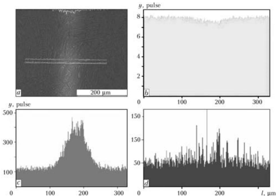
**Figure 3.** Microstructure of seam metal (*a*), and quantitative distribution of titanium (*b*), zirconium (*c*) and cobalt (*d*) over the width of brazed joint along scanning line (OT4 base metal, Ti-Zr-Co BFM)
