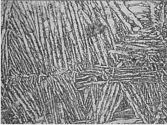
**Figure 2.** Microstructure ( $\times 500$ , light microscope) of central area of seam of brazed joint (OT4 base metal, Ti-Zr-Co BFM)
