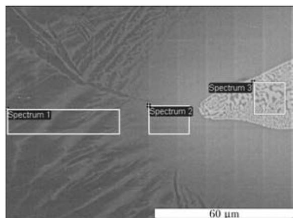
**Figure 5.** Microstructure and near-fillet areas of X-ray microspectrum analysis of brazed joint (OT4 base metal, Ti-Zr-Fe BFM)
