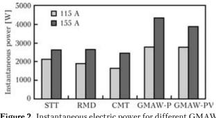
Figure 2. Instantaneous electric power for different GMAW processes
