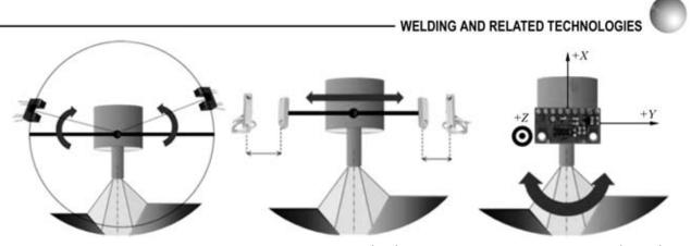
Figure 6. Sensors used in Conparte system: magnetic 9028PA (*left*), optic infrared receiver TCST1103 (*center*) and accelerometer MMA7361L (*right*)
