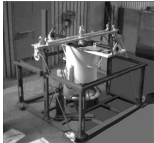
Figure 20. Module for joining the damaged pipes of wells
