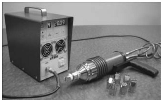
**Figure 5.** Advanced compact equipment for UIT/UP of materials, parts and welded elements
