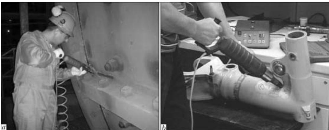
**Figure 8.** Examples of application of the UltraPeen system for fatigue improvement: a – of grinding mill when over 250 m of welds were treated; b – of landing gear where critical from the fatigue point of view zone was treated
