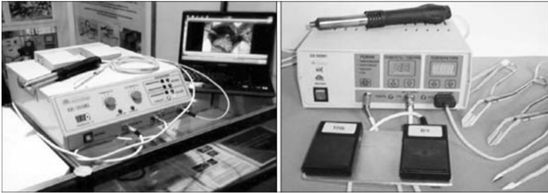
Figure 17. Multifunctional apparatuses for high-frequency welding and CI-treatment of live tissues, based on EK-300M1
