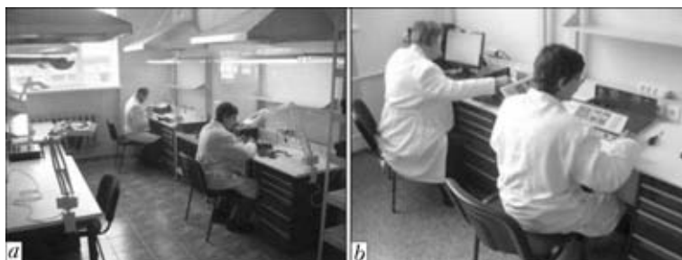
Figure 2. Area for manufacturing HF LTW apparatuses at STC «E.O. Paton Electric Welding Institute»: a – incoming inspection and setting-up of elements and components; b – apparatus assembly and programming
