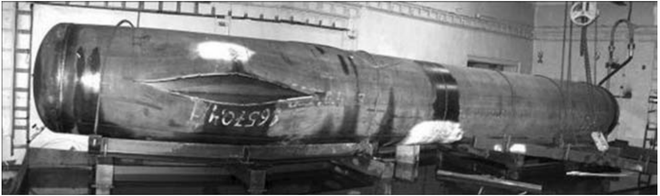
Figure 4. Stand for service life tests of pipe elements of up to 6 m length
