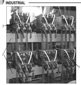
**Figure 1.** Appearance of welding machines ASh-110 assembled into blocks: 1, 3 — working and doubling welding machines, respectively; 2 — traverses for fastening the machines
