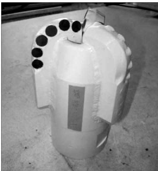
**Figure 4.** Appearance of bit blade with brazed-in DHC
