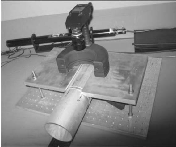
**Figure 3.** Device and specialized fixture for measurement of residual stresses of welded circumferential joints of AMg6 alloy using method of speckle-interferometry
