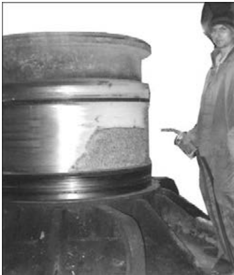
Figure 1. Surfacing of mill journal by semi-automatic welding machine and journal draft
