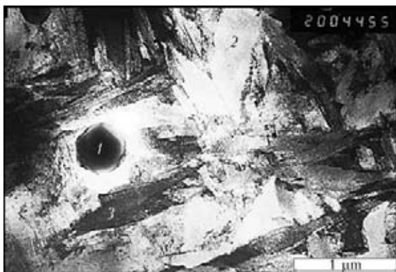
Figure 4. TEM-microstructure ( \times 20000 ) of base metal of sample from R6M5 steel: 1 – carbides; 2 – residual austenite; 3 – tempering martensite
