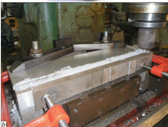
Figure 8. View of tool made from steel P18 (a), and FSP of surface layer of ML10 alloy block (b)
