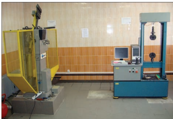
Figure 8. Rupture machine R5M and pendulum hammer 2010 KM-30
