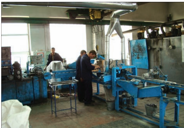
Figure 6. Line of manufacture of electrodes in press PEO 1000
