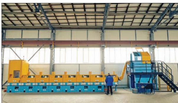
Figure 3. New technological line for manufacture of copper-plated welding wire
