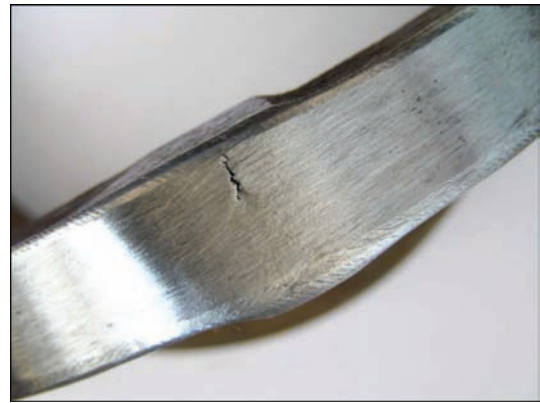
Figure 6. Appearance of specimen with a crack along the welding line
