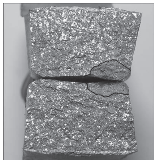
Figure 7. DS at the fracture surface
