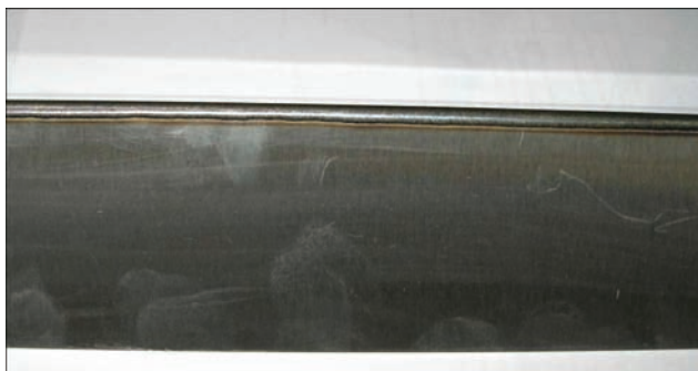
Figure 7. Welded specimen of fillet joint without temper colors after argon arc welding in automatic mode
