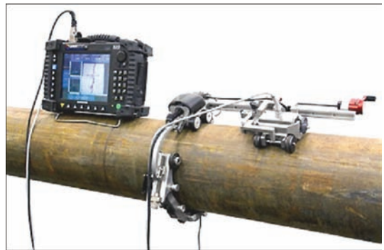
Figure 2. Mechanized system of ECT of pipes
