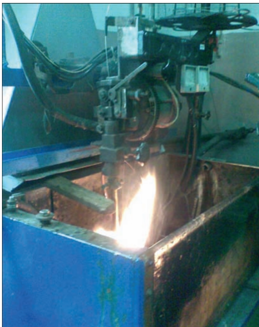
Figure 1. Welding with coolant FXC2
