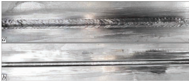
Figure 9. Butt joint of 1561 alloy ( \delta = 5 mm) produced by hybrid Plasma-MIG welding in the developed robotic complex: a — upper bead; b — lower bead
