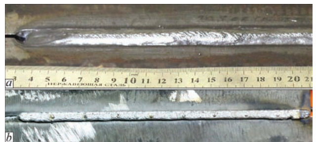
Figure 8. Butt joint of steel 20 ( \delta = 20 mm), produced by hybrid Plasma-MIG welding in robotic complex; a — upper bead; b — lower bead
