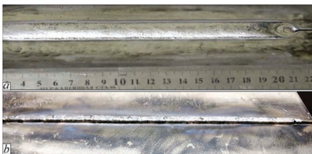
Figure 7. Butt joint of SUS304 steel ( \delta = 12 mm), produced by hybrid Plasma-MIG welding in the developed robotic complex: a — upper bead; b — lower bead
