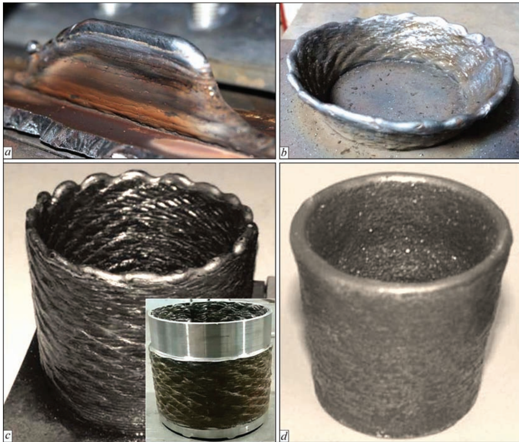
Figure 6. Metal products, manufactured in the developed complex: a — 5×70 mm wall; plasma surfacing with Sv-08G2S wire (1.2 mm diameter) in 50 passes; b — cone, surfacing with Sv-08G2S wire (1.0 mm diameter); c — 80 mm diameter sleeve, MIG/MAG surfacing with Sv-08G2S wire (1.2 mm diameter); d — 40 mm diameter sleeve, microplasma surfacing with PG-10N-04 powder
