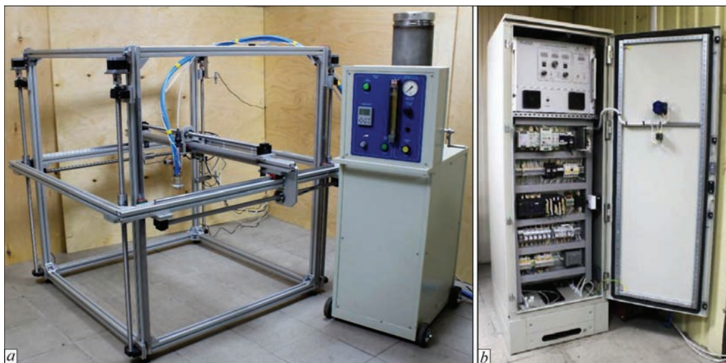
Figure 5. Automated complex for additive surfacing of bulk metal products: a — manipulator with plasmatron and powder meter-feeder; b — appearance of power and control block with open face panel
