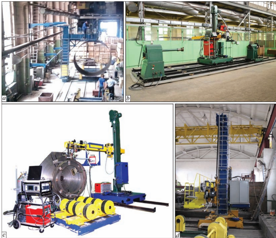
Figure 3. Complexes of automation and mechanization of welding processes with use of special MWE
