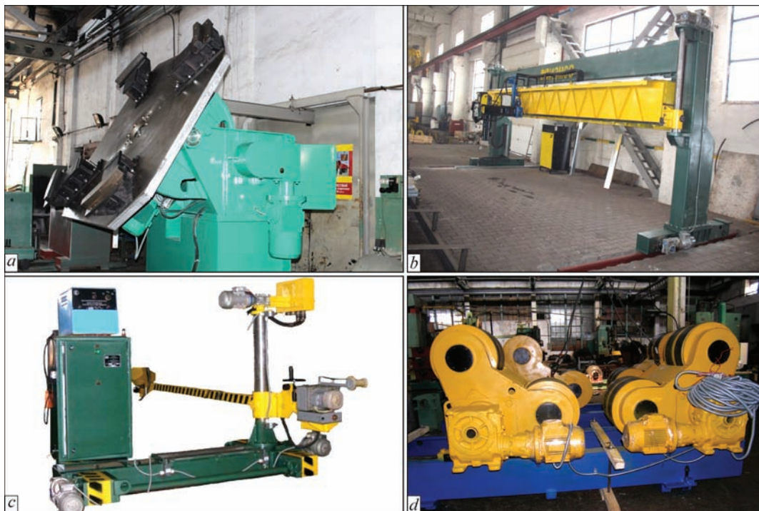
Figure 4. Unique models of MWE: universal manipulator of 7000 kg loading capacity (a), moving gantry (b), installation for semi-automatic submerged arc welding of circumferential and longitudinal inner welds (c), balancing rotator with a load capacity of 40000 kg (d)
