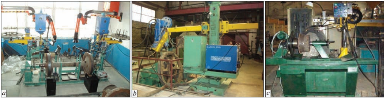
Figure 1. Installations for surfacing and restoration of parts: RM-09 (a); RM-15 (b); IZRM-05 (c)
