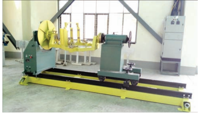
Installation for assembly and welding of suspended tanks
