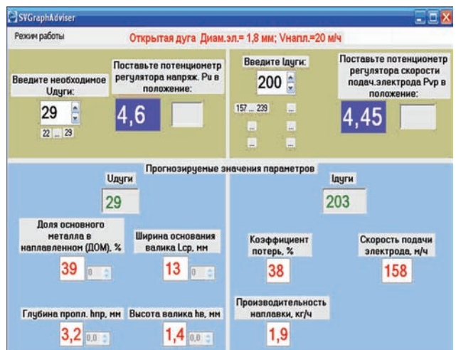
Figure 4. View of computer screen with preset modes of open arc surfacing by flux-cored wire of 1.8 mm diameter and predicted characteristics of surfacing process and geometric dimensions of deposited beads
