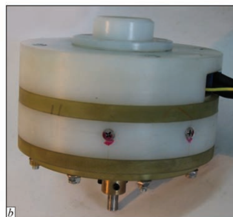
Figure 2. Electrode device for EDT: a — schematic diagram ( l — electrode; 2 — body; 3 — disc; 4 — inductance coil; 5 — cover; 6, 7 — terminals); b — appearance
