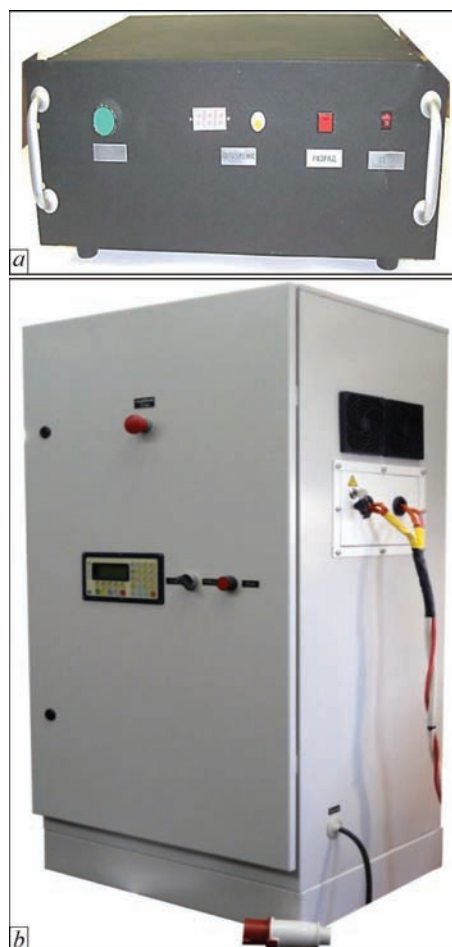
Figure 1. Appearance of single-circuit ( a ) and double-circuit ( b ) sources of pulsed electric current for EDT
