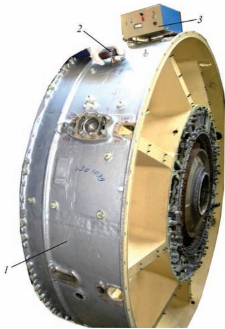
Figure 18. Treatment of repair weld on the outer surface of the outer shell of IBAE of the ML10 alloy applying EDT method: 1 — IBAE; 2 — electrode device; 3 — power source for EDT
