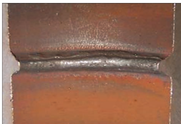
Figure 4. Welded joint formation in MIABPW
