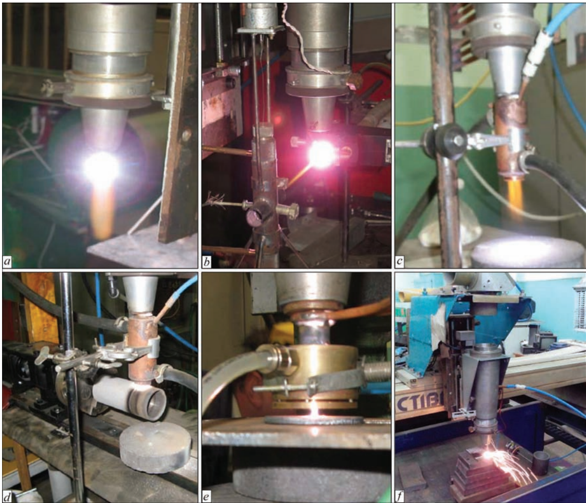
Figure 1. Laboratory stands for investigation of COD technological capabilities: a — COD, running in an argon jet, in atmosphere; b — hybrid interaction of COD and microplasma; c — plasmatron operating on COD base in nitrogen; d — treatment of bodies of revolution with COD; e — hybrid plasmatron with COD pumping by DC arc; f — COD surfacing
