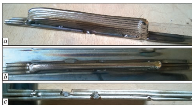
Figure 6. Sample produced using wire as deposition substrate: a — side view; b — top view; c — bottom view
