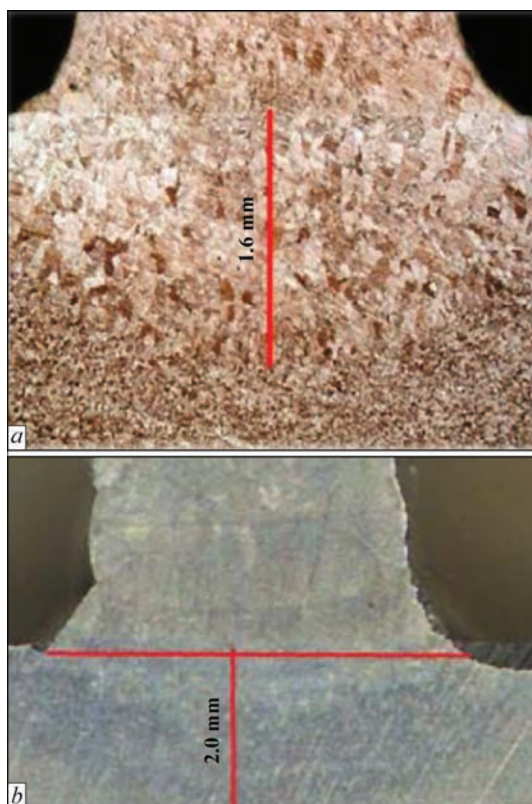
Figure 5. Macrosection of HAZ metal at wire deposition: a — 1.6 mm VT1-0 titanium wire on VT1-0 titanium plate; b — 3 mm Ti-6Al-4V titanium alloy wire on Ti-6Al-4V alloy plate
