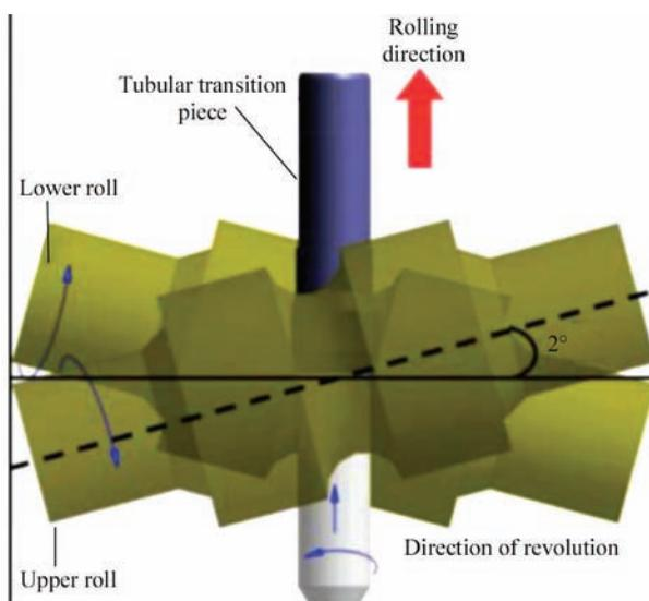
**Figure 2.** View of roll positioning and directions of motion during rolling (*top view*)
