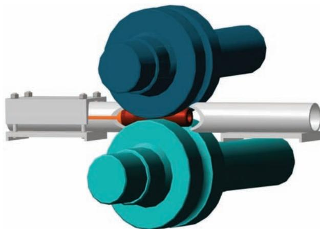
**Figure 5.** Positioning of grooved rolls with guides
