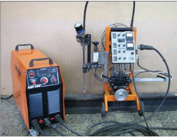
Figure 1. Set of pilot equipment for automatic arc surfacing of rails with flux-cored wire
