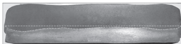
Figure 3. Macrosection of bimetal sample (25M experiment). Dotted line denotes metal mixing zone
