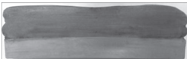
Figure 3. Macrosection of bimetal billet from experiment 45M
