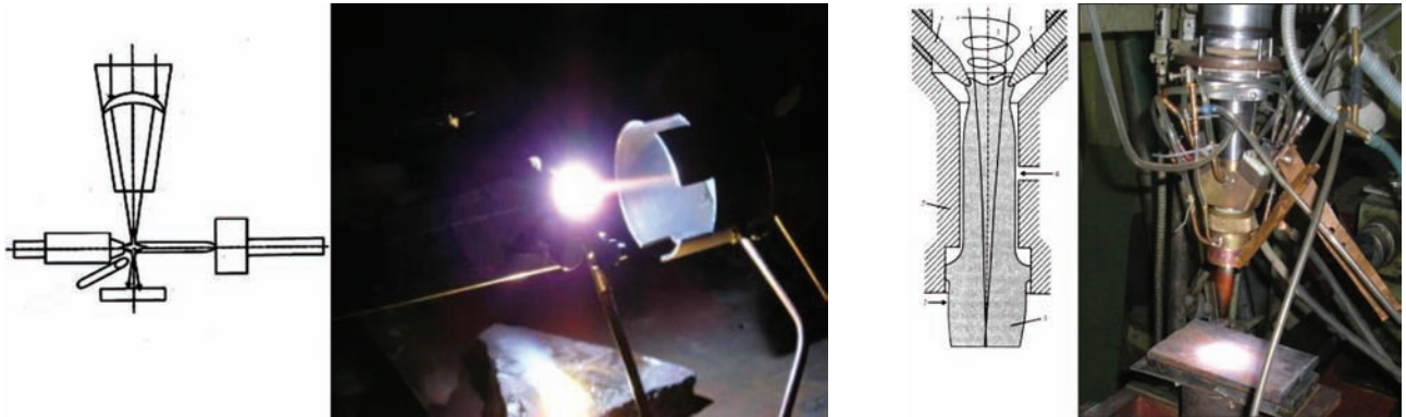
Intercoupling of plasma jet with laser radiation: CO 2 -laser (2 kW), plasmatron MP-03 (2 kW)
