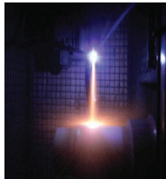
Process of plasma-arc spraying with current-carrying wire
