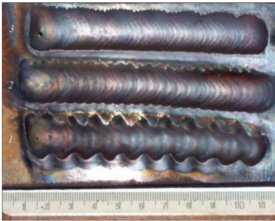
Figure 4. Appearance of beads deposited by plasma-powder method with plasmatron oscillation at frequency, \text{min}^{-1} : 1 — 40; 2 — 60; 3 — 90) amplitude of oscillations — 10 mm)
