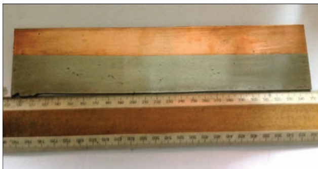
Figure 8. Template of steel-copper plate (thickness of copper layer 40 mm)
