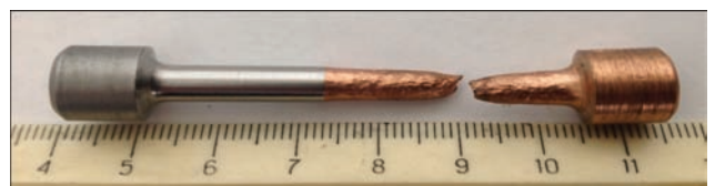
Figure 9. Sample after static tension test
