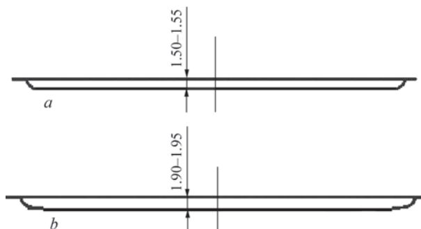
Figure 2. Boundary of T_m isotherm in the plane normal to the processed surface (45×0.7 mm strip): a — deposition on steel 25Kh1M1F; b — on sublayer from steel 08Kh17N12M2
