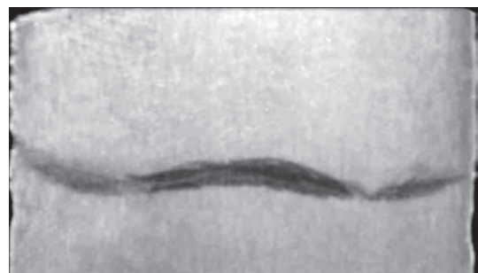
Figure 3. Shape of metal pool in the metal surfaced, formed during electroslag remelting (surfacing) of discrete filler in the CSM
