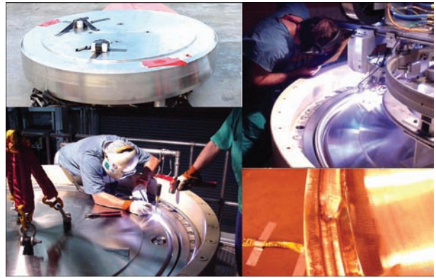
Figure 4. Welding-up of canister lid
