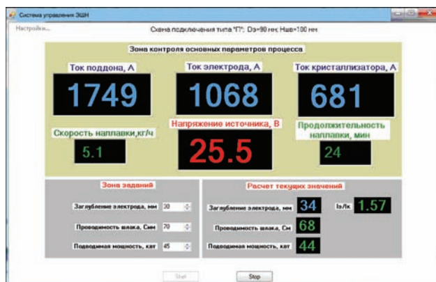
Figure 7. Appearance of computer screen during system operation in control mode, regulation and registration of surfacing process
